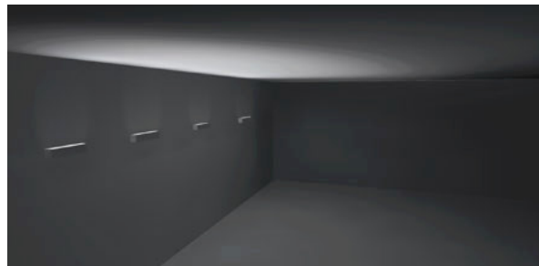
W-shaped light distribution Optical simulation with a distance of 0.7m between lamps and a height of 1m from the ceiling
